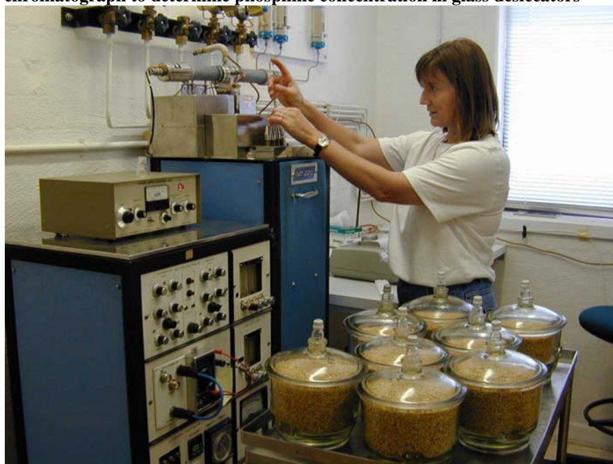
Figure 1: Gaye Weller of CSIRO Entomology performing the small-scale fumigations using gas chromatograph to determine phosphine concentration in glass desiccators
